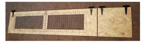
12) Reattach the doors. Fit 3 hasps and staple fasteners, 2 or 3 for the mesh door and 1 for the bedroom door. Screw the hasp to the top (E) using 1x 30mm screw and the staple to doors (I) and (J) using 4x 12mm screws. Secure the fastener with a wooden peg through the staple loop.
