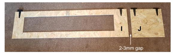
Once hinges are attached, the doors can be attached to the bottom of the main hutch (panel B) ensuring there is a 2 to 3mm gap between the doors so they don't catch on each other.
