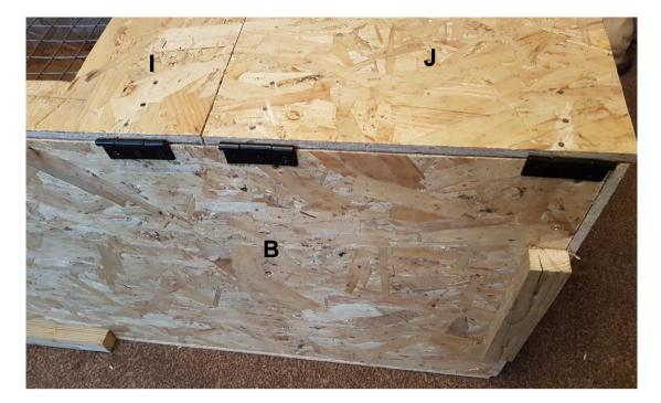
10) Cut out the opening in door (I) for the mesh. With the door attached and closed (which makes it easier to do this next step), measure 7cm in from the top and bottom and 13cm from the sides and draw a rectangle. You can either cut one opening (2a) or cut two openings with a 8cm centre post for added strength (2b). Drill an 8mm hole in each corner, then using a jigsaw cut out the opening(s).
