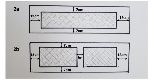
11) Remove the door for the next process. Lay the mesh over the opening(s) and mark the mesh with a 3 to 4cm overlap all the way round. Trim the mesh using heavy duty scissors or wire cutters/tin snips. Staple with a cable stapler or hammer 10mm U nails every 3 to 4cm ensuring the mesh is on the inside of the door. Make sure any sharp edges are made safe so hedgehogs do not injure themselves.
